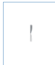
Stylus tip 33 mm Order no.: 101-011-330 made of carbide, \varnothing 3.5 mm / R: 25 \mu m / A: 12° with optaDiamond coating
