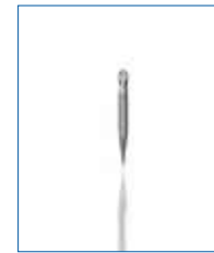
Stylus tip 59.5 mm conical Order no.: 101-110-595 made of carbide, \varnothing 3.5 mm / R: 25 \mu m / A: 24°
